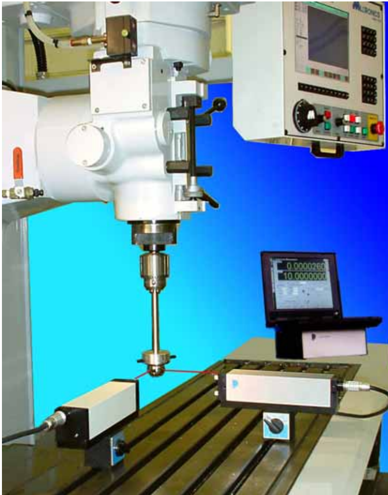
Fig. 11-2 A Photo of a Typical Setup for the Measurement of Spindle Error Motion
